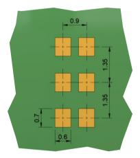
Recommendation: Solder paste mask: 0.2mm smaller than footprint Solder mask expansion: 0.05mm Stencil thickness: 100um
