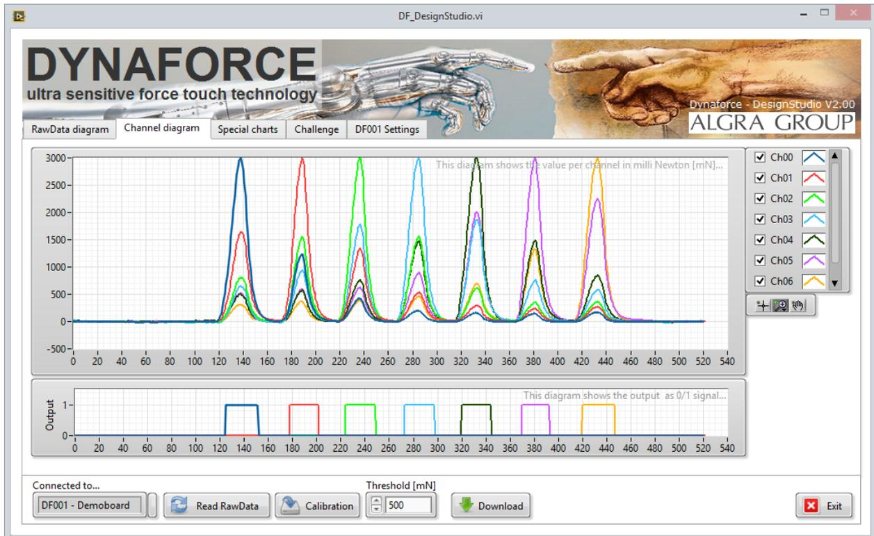
After calibration, the calibrated sensor values are visualized in the upper graph of the tab *Channel diagram*. In the lower graph, the corresponding digital output signals are plotted.
